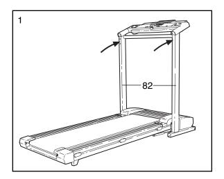
2. Remove the Lock Knob (110) from the Lock Pin (114).
